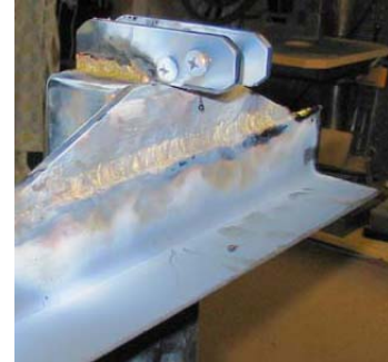
The clamp mounts, after they've been brazed on
