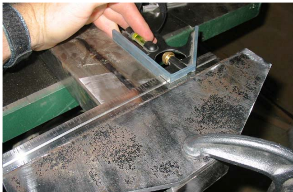
Squaring the torsion plate to the tubing (Note that the prototype in the picture doesn't have a spacer plate)
