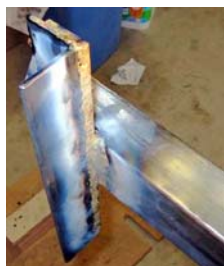
Squaring the torsion plate to the tubing (Note that the prototype in the picture doesn't have a spacer plate)
