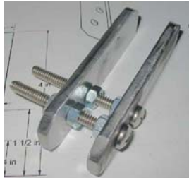
Use a couple of long 1/4" bolts and some nuts to keep the plates the right distance apart
