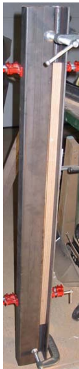
Clamping the angle-iron and tubing together. (Note the wooden spacer)
